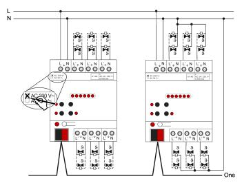
Figure 3: Connection for AC 230 V actuators (connection examples)
